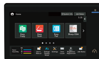
10.1" (diagonally measured) customizable touchscreen display.
